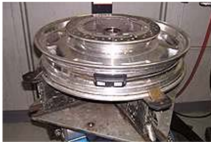
Transmitter mounted on wheel rim using very long hose clamp. Installation courtesy of All Cycle Sales, Tempe, AZ.
