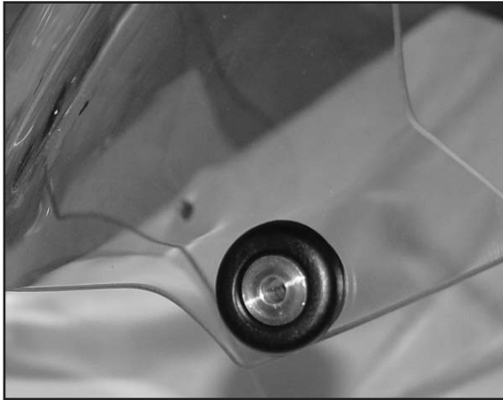
Figure 4 Showing Exterior Bushing
